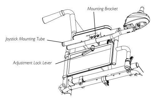
FIGURE 9.1 Preparing the Joystick for Use
